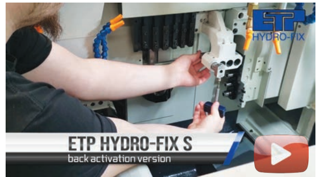
Back activation version in Drill arm application. Tool change in 30 seconds!
